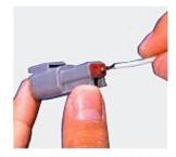
3. Push contact straight into connector grommet until a click is felt. Slightly tug to confirm that it is properly locked in place.
