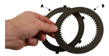
3. Alternate between the outside tabbed and inside splined discs with the friction side up.
